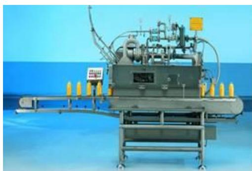
After filling, the containers should be moved to the **sealing process** by the **shortest route**, in order to avoid unnecessary **loss of temperature** and to minimise the risk of **contamination** of the filled product by foreign substances or any airborne bacteria. Apart from **manual capping**, which is hardly used on an industrial scale, Twist-Off® closures are mostly capped automatically by means of **straight line sealing machines**.
